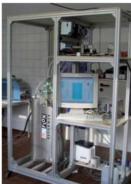
Erdgas-Wasserstoff-Dampfreformer Natural gas hydrogen steam reformer
