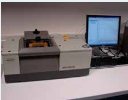
Infrarotspektrometer zur CO 2 Messung Infrared spectrometer for CO 2 measurement
